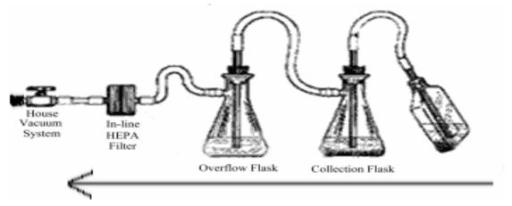
The filter should be replaced whenever there is evidence of filter failure or blockage, and, on a routine basis (no less often than annually). Filtering devices are available commercially via Fisher (Whatman Vacu-Gard <sup>™</sup>).
