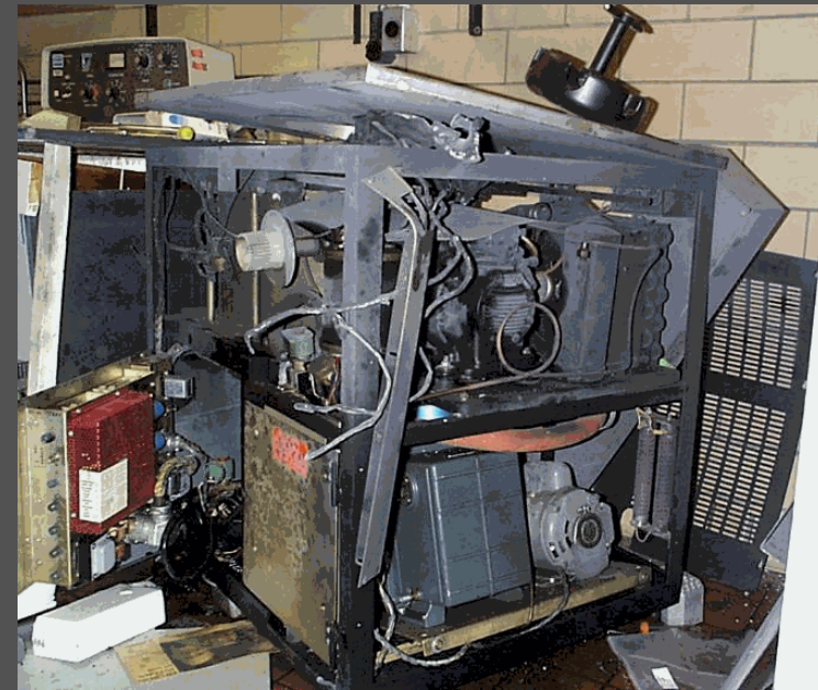
Ultracentrifuge destroyed by broken spindle (AIHA)
